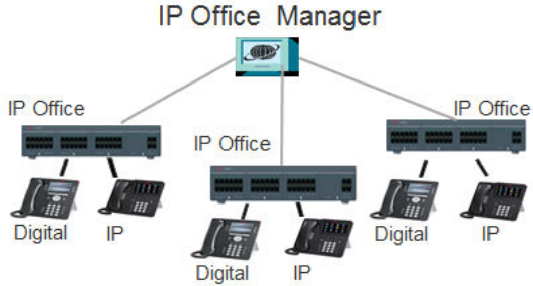
Figure 1: IP Office systems connected to a single IP Office Manager endpoint
